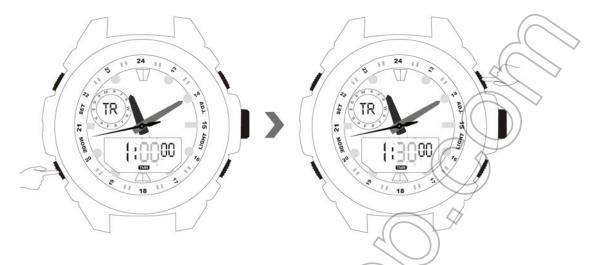
5.2.3 Press the "Mode" button again to move the flashing to the seconds setting. While it is flashing, use the "ADJ" button to change it.
