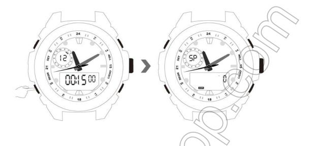
3.2 Press the "ADJ" button while in the Stopwatch Mode to start the stopwatch.
